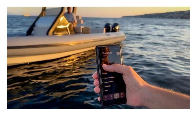
KYMS comprises an onboard embedded system, a cloud platform, and web/mobile applications. It acquires information through the NMEA2000 network, covering aspects like engine data, GPS, radar, and more. It assists operators in navigation and docking,
