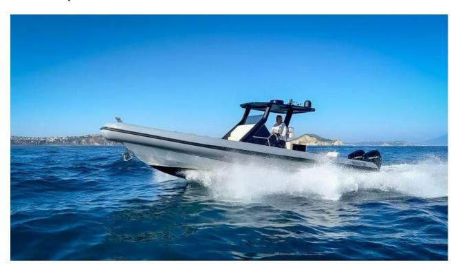
Equipped with a pair of 225 HP outboard Mercury engines, it can reach speeds exceeding 40 knots, with cruise consumption of between 20 and 30 knots below 2.5 liters per mile. It is a trailerable inflatable boat thanks to its maximum width when deflated of 2.5 metres.
