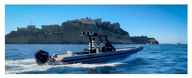
Equipped with a pair of 225 hp outboard mercury engines, it can reach speeds exceeding 40 knots, with cruise consumption of between 20 and 30 knots below 2.5 liters per mile. It is a trailerable inflatable boat thanks to its maximum width when deflated of 2.5 metres.
